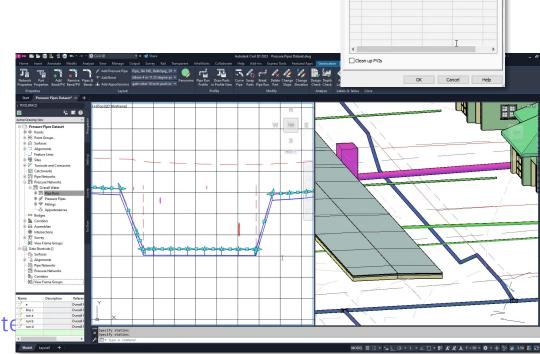
Assign offset preferences along a station range of a pressure pipe profile.
